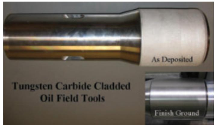
Fig. 11 — Oil field component clad with wear-resistant tungsten carbide alloys.
