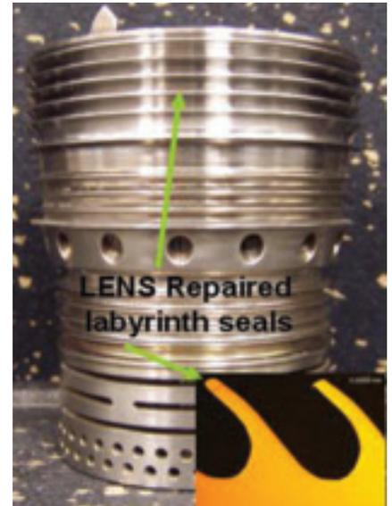
Fig. 4 — Repair of Inconel® 718 compressor seal.
