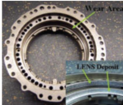
Fig. 3 — Low-wattage repair of Ti-6Al-4V bearing housing.
