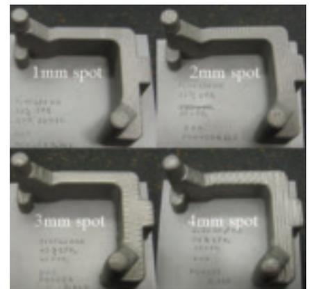
Fig. 7 — Freeforms of 316 stainless steel at various parameters.
