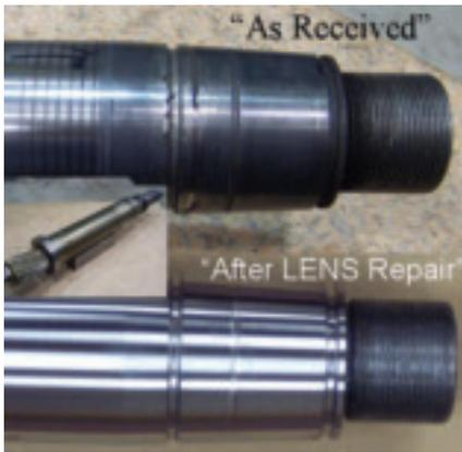
Fig. 5 — Comparison of thermal spray repaired (top) shaft and LENS® repaired shaft.
