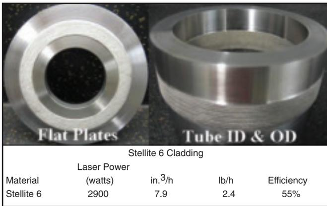
Fig. 10 — Cladding projects of #6 Stellite®, which includes thrust surfaces and inside and outside of bearing/bushing.
